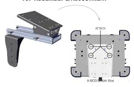
3. Pull the rear knob to release and move the top assembly. Slide it forward to the front locating knob and it will automatically lock in position. From this point you will be able to mount A-MOD Desktop/docking equipment to the top plate via holes and slots from the underside with provided 1/4"-20 bolts and washers.
