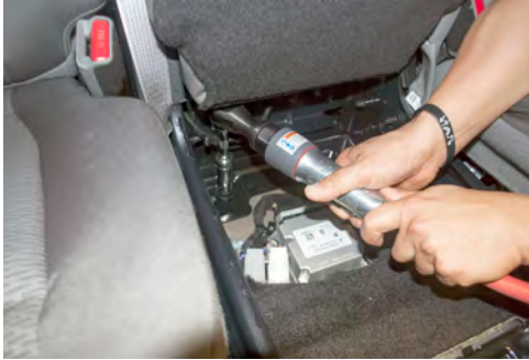
Remove (2) 18mm bolts from the rear of the OEM center seat.
