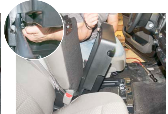
Lift the plastic base from the center console, being careful to disconnect the wires from the rear of the base.
