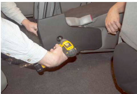
Remove rear bracket from OEM sea, held in place by (3) 1/2" bolts. Reinstall OEM bracket back into vehicle re-using (2) OEM 18mm bolts, that were removed 3 steps earlier.
