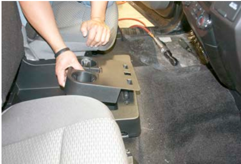
Lift up center console and remove OEM cup holder and set aside.
