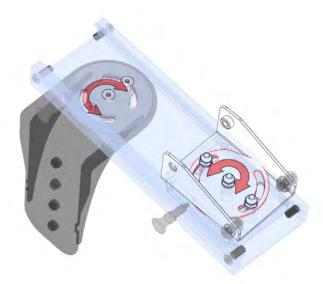
4. The swivel tension to the Motion Arm and Tilt/Swivel Assembly is set at the factory. This can be adjusted by loosening and/or tightening the (3)  $\frac{1}{4}$ "-20 nuts at each location. Use a  $\frac{1}{16}$ " wrench to stabilize the nut and a  $\frac{5}{32}$  T-handle hex key to turn the bolt.
