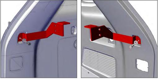
Secure the Driver Side and Passenger Side Front Support Brackets with (2) ¼-20 x ¾ Bolts and Washers.
