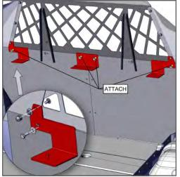
5. Attach the Driver Side, Center, and Passenger Side Rear Support Brackets with (4) ¼-20 x 3/4 Bolts and Washers. Secure the upper mounting holes of the Driver Side and Passenger Side Support Brackets on top of the Upper Poly Wings with the previously removed hardware.
