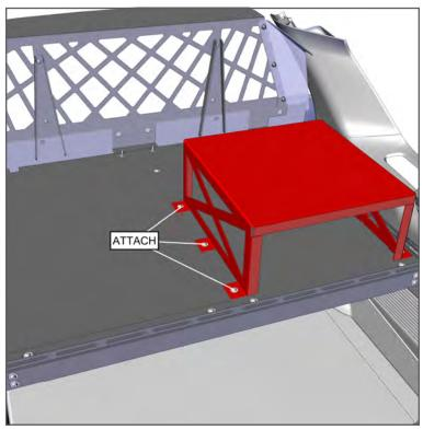
9. After equipment is secured to the Equipment Tray, attach the Equipment Cover with (6) 1/4-20 x 5/8 Socket Head Cap Screws and Washers.
