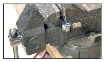
Use 9/16" box end wrench to secure the flange nut. 4.
