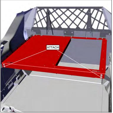
7. Insert the Cargo Cover into the vehicle resting on top of the Front and Rear Support Brackets. Secure the front of the Cargo Cover to the Front Support Brackets with (4) 1/4-20 x 5/8 Button Head Cap Screws and Washers.
