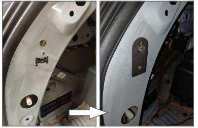
Drill or pop out the OEM mounting clip that held the Jig in place. Install AVK fastener and attach the Driver Side and Passenger Side D-Pillar Straps. Replace OEM trim.
