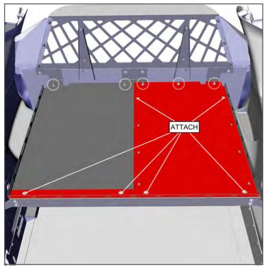
8. Insert the removable Equipment Tray and Edge Bracket. Secure to the Cargo Cover with (6) 1/2-20 x 5/8 Button Head Cap Screws and Washers, and to the Rear Support Brackets with (5) Flange Nuts.
