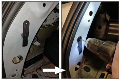
Use the previously removed OEM screw to attach the drill template (Jig) to ensure proper placement of the AVK fastener. Be sure the Jig is perfectly vertical before drilling 1/8" pilot hole followed by a 25/64 finished hole.
