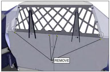
4. Remove (4) ¼-20 Socket Head Cap Screws attaching the Cargo Cover to the Top Bar and the lower mounting hardware securing the Driver Side and Passenger Side Poly Wings.
