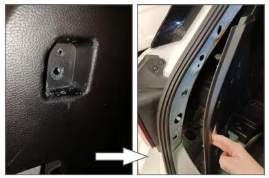
1. Unscrew the (2) OEM Trunk Cargo Net Tie-Down Hooks and pop loose the D-pillar trim. Drill OEM trim mounting hole to 9/32'.
