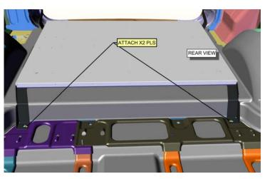
Loosely attach the left and right rear feet to the Base Insert Platform Unit into vehicle. Secure the
