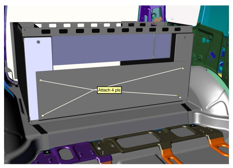
Attach Backstop onto Storage System using (4) Button Head Cap Screws.
