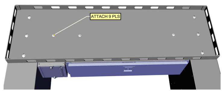
Set Package Tray on top of rear of Towers and/or Horizontal Drawer. Secure into place using (8) Buttonhead Cap Screws (\*use (6) Buttonhead Cap Screws if purchased without Horizontal Drawer).
