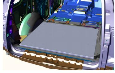
Once Base Assembly is placed into the vehicle, Install adhesive Foam Pads for noise reduction on check to make sure all hardware is tight and secure. the inside of the Small Box.
