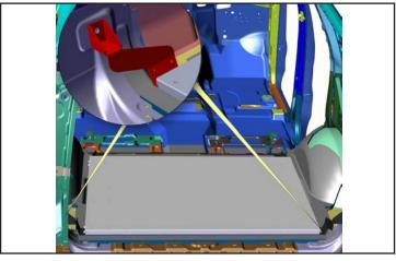
Attach the Front Brackets with the provided 1/4-20 Secure the Front Bracket to the vehicle with the previously removed bolts.
