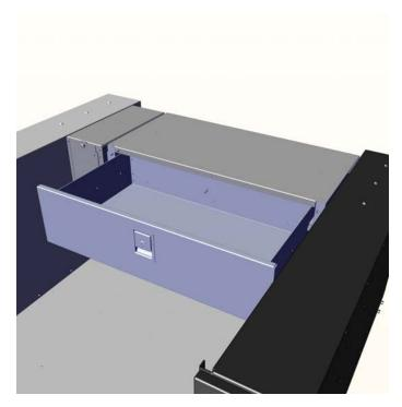
Holding Drawer for easiest view and access, place a Button Head Cap Screw and washer through rear top hole opening. Loosely secure to thread hole of Tower, then rotate Drawer into proper position and place a Button Head Cap Screw and washer through front top hole opening, secure to threaded holes of Tower.
