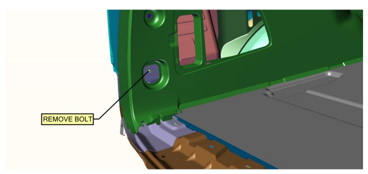
Remove factory OEM bolt with a T-40 Torque Socket on the left and right side of the vehicle. Set aside for assembly.
