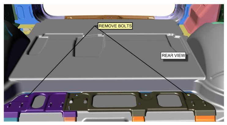
Remove the (2) OEM back inside rear seat bolts with an 18 mm socket.
