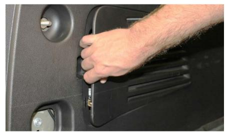
Remove Jack Location Panel, the Wheel Chocks, and the Jack from its location. Place the Jack Location Panel back in its original location once the Wheel Chocks and Jack have been removed.
