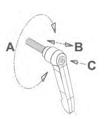
**NOTE:** Insert the ratchet handle through the unthreaded side of the articulated swing arm and tighten. Going through threaded side first will not allow the arm to tighten properly
