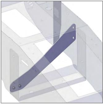
Loosely attach the Cross Brace to the Consoles front lower support Mount Bracket with (2) 1/4"-20 bolts.
