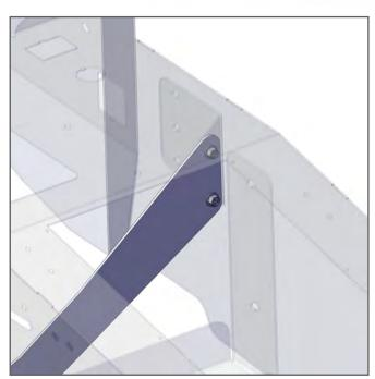
Attach the Stiffener Plate to the upper side of the Cross Brace with (2) 1/4"-20 bolts.
