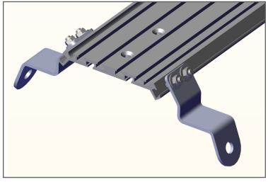
Once the Floor Plate is installed, adjust the floor plate (front to rear) as needed. Tighten the 5/16 nuts securing the legs with a ½" socket.
