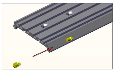
Install (8) of the 5/16-18 bolts in the side channel of the Floor Plate, four per side.
