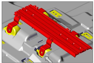
Align the Floor Plate Legs with the holes in floor board. Replace with OEM hardware
