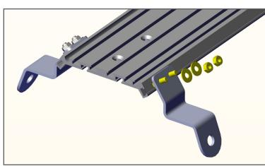
Line up the bolts with the holes in each leg and secure with the provided 5/16 washers and 5/16 nuts. Lightly tighten so that adjustment will be easier after installed in the vehicle.
