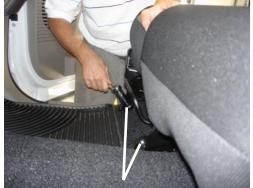
Remove the 2 front seat bolts from the passenger side seat.
