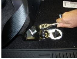
Remove the center console bolt using a T55 Hex Head.
