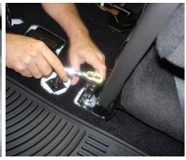
Remove the center console bolt and now remove console.
