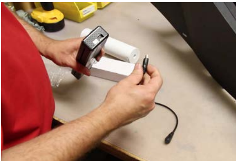
A 6 foot USB/Micro to USB cable is included. Secure one end into Brother printer and the other into the computer USB port.
