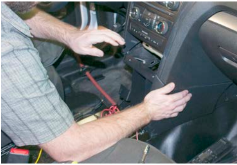
Replace OEM Trim Panels, securing to provided Dash Mount Structure.
