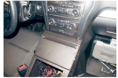
Place Jotto Desk Contour Console into the vehicle dash area...lining up the Dash Mount Bracket to the Middle Dash Structure. Loosely secure using provided hardware.
