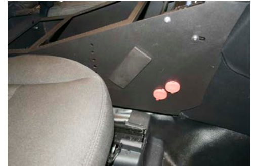
Mount USB/Line-in plate into Contour Console. Attach the wiring for the provided 12V outlets, and re-attach USB/line-in.
