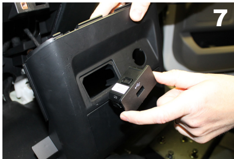
Relocate USB into storage box of Contour Console. Snap USB port into Console. Plug in USB cable.
