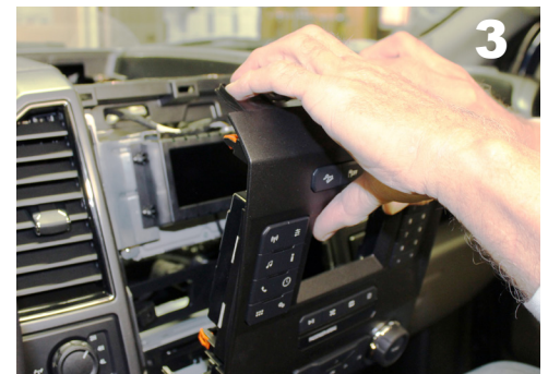
Pry from the top to unsnap the trim covering the radio and climate controls. Unplug the heater control from the harness.
