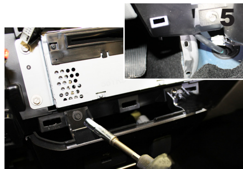
Remove lower panel containing 12 volt power and USB by unscrewing (2) 7mm screws on the top and (2) 10mm screws on the bottom. Unplug accessories from harness.
