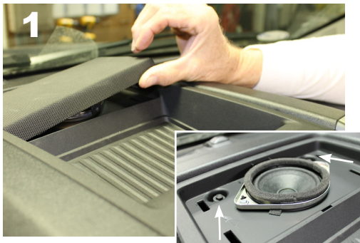
Unsnap speaker cover from each side corner to remove (2) 7mm screws.
