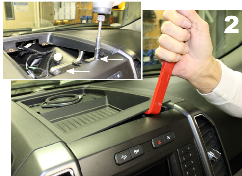
Pry the top tray up from each front corner and remove the (2) 7mm screws. Unplug speaker from the harness.
