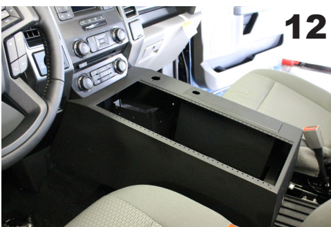
Place Console on Floor Plate making sure Console slides up against the dash and secure in place.
