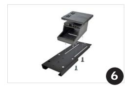
Outside of vehicle insert 4 carriage bolts through bottom of plate. Align console slots onto carriage bolts and finger tighten with provided nuts.
