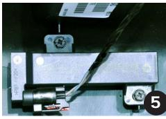
Remove Ignition Proximity Sensor from plastic OEM console. Ignition Proximity Sensor should be remounted onto top of transmission hump with Velcro or double sided tape.
