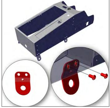
Outside of vehicle, loosely attach Rear Legs, Front P/S, and Front D/S Legs with provided hardware. Install Contour Console into the vehicle from the rear seat area, sliding forward until mating up with OEM dash structure.
