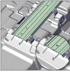
Slide (4) 5/16-18 bolts into the top, outside mounting slots of the Floor Plate to secure the Console.
