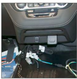
Remove 110V outlet from OEM dash trim. USB/ SD will be on 3' cable under P/S seat.
