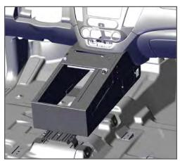
10. Adjust the Console by moving it forward and back along the Floor Plate. Move the Console to the nesting position along the dash, secure by tightening all hardware.
