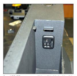
USB/SD connector will install inside locking lid of Jotto Desk Contour Console. Press connector until it securely snaps into place.
