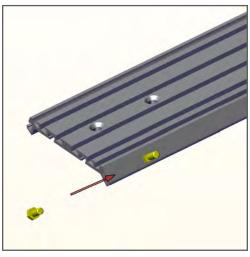
2. Install (8) of the 5/16-18 bolts in the side channel of the Floor Plate, four per side.
