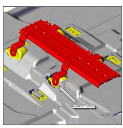
4. Align the Floor Plate Legs with the holes in floor board. Replace with OEM hardware or provided self-tapping bolts.
