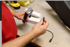
A 90° USB/USB extension cable is attached to the paper roll rod. Secure one end into Printek Mobile 180 or Brother PJ6/7 printer and the other into the USB cable.
