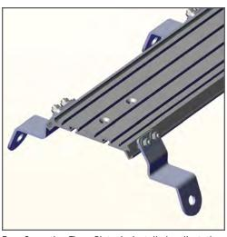
5. Once the Floor Plate is installed, adjust the floor plate (front to rear) as needed. Tighten the 5/16 nuts securing the legs with a ½" socket.
