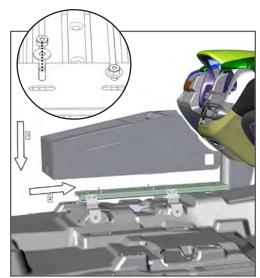
. Set the Console on the Floor Plate. Align the bolts with the mounting slots of the Console Mounting Bracket. Add the washer and nuts - \*snug, do not tighten\*.
