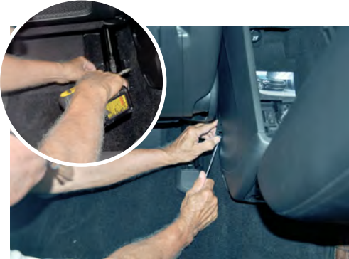
Move seats forward, use a flat head screw driver to expose and then remove (2) 10mm bolts.
