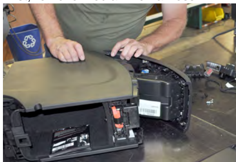
Now pry rear OEM cover from console.
