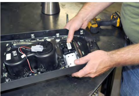
Traction switch/coin tray will pop out from underside of OEM console. Set aside.
