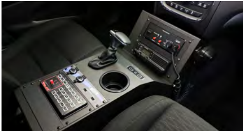
Traction switch/coin tray will install into faceplate opening.
