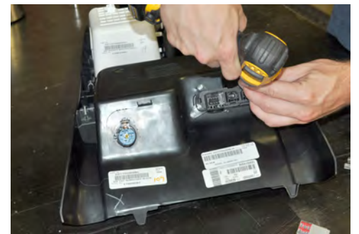
Using a T20 bit, remove (4) screws and set aside media component to remount into Contour Console.
