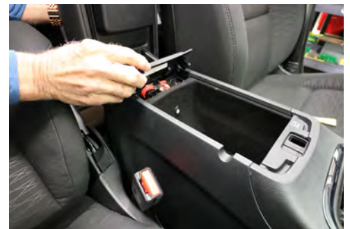
Pry up manual neutral cover located under armrest near the hinge.
