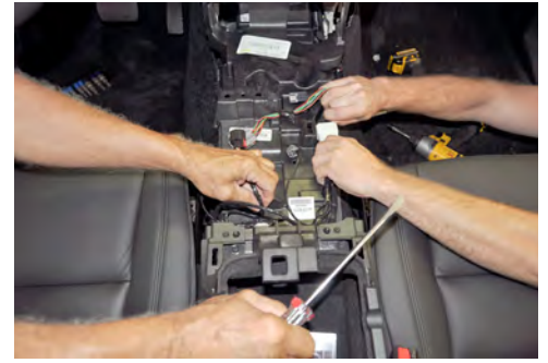
Disconnect wiring harnesses and harness clips.
