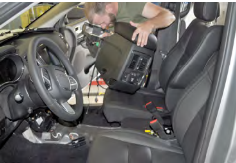
Remove OEM console from vehicle.
