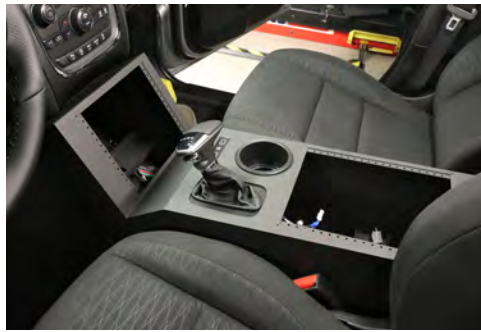
Install Jotto Desk Contour Console using 5/16 button head cap screws.
