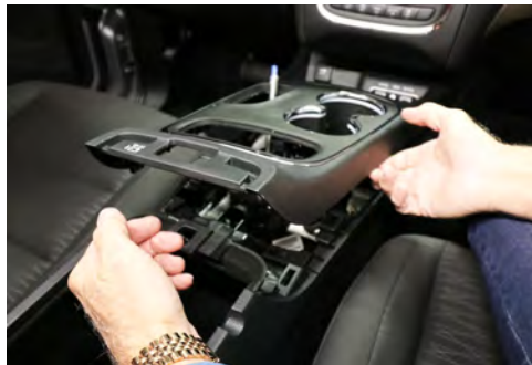
Pry up top/center OEM console. Disconnect all wires from top cover.
