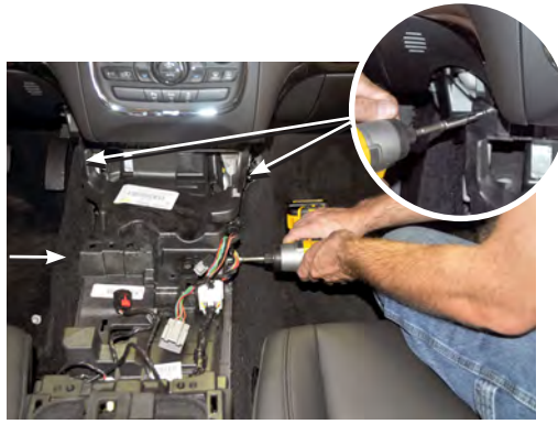
Remove (2) 10mm bolts and (2) 7mm bolts.
