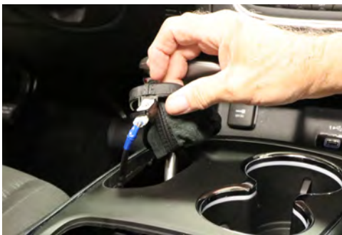
Pop up shifter boot. Unscrew bolt on shifter with T20 bit and unplug wire cord.
