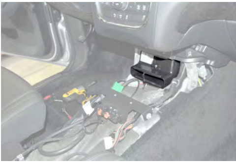
Install foam insert into open duct.
