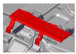
Align the Floor Plate Legs with the holes in floor board. Replace with OEM hardware.
