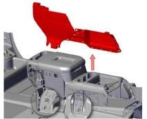
Unsnap side trim from left and right of center console exposing center console OEM bolts. Remove center console.
