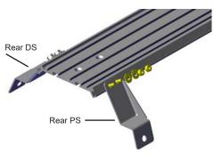
Line up the bolts with the holes in each leg and secure with the provided 5/16 washers and 5/16 nuts. Lightly tighten so that adjustment will be easier after installed in the vehicle.
