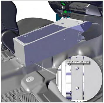
4. Place Durango IPB Contour Console into vehicle. Secure the previously attached Front Mounting Tabs of the Console with previously removed OEM hardware, and the rear of the Console to the Console Mount Bracket with provided socket head cap screws.
