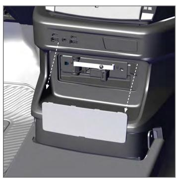
1. Remove the trim exposing the Manual Park Release (MPR). With the trim removed and Console installed, this will make access easier by only removing one Console Faceplate/Radio.
