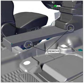
2. Remove (4) OEM bolts and retain for later use. Set OEM Floor Plate aside.
