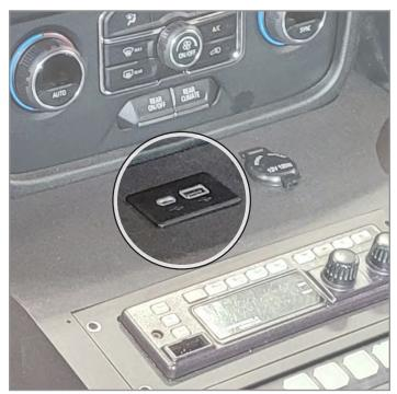
4. Relocate OEM USB/Line-in housing to Contour Console and re-connect previously removed cables.
