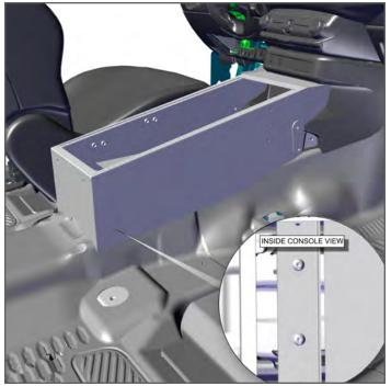
4. Place Durango Contour Console into vehicle. Secure the previously attached Front Mounting Tabs of the Console with previously removed OEM hardware, and the rear of the Console to the Console Mount Bracket with provided socket head cap screws.
