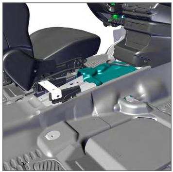
3. Attach the Console Mount Bracket with previously removed OEM hardware to the rear OEM Floor Plate mounting points.
