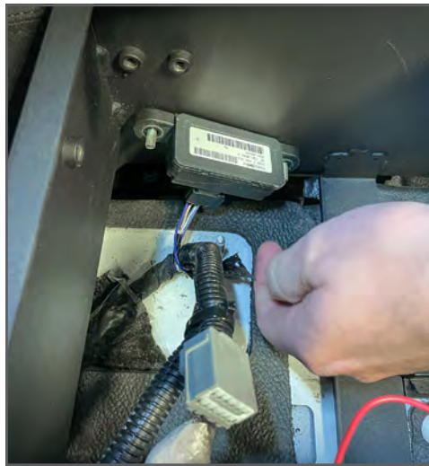
10. Plug in and relocate the Proximity Sensor to the mounting studs in the Console with previously removed OEM flange nuts. You can now relocate the OEM 12v outlets and plug in OEM harness.
