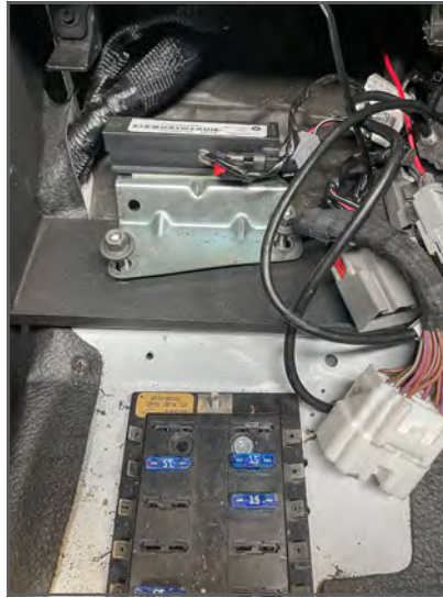
7. Insert the Console into the vehicle. Pull the previously unplugged harness in-between the Consoles Center Mounting Supports. Slide the Consoles front Mount Support under the sensor plate.
