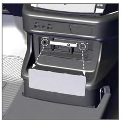
1. Pop loose the trim and remove exposed hardware securing the Manual Park Release (MPR) to the lower Dash Structure.
