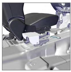
Attach the Rear Console Mount Bracket with previously removed OEM hardware to the rear OEM Floor Plate mounting points.
