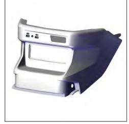
Pop loose and remove the lower OEM dash structure from the vehicle. Set Aside.
