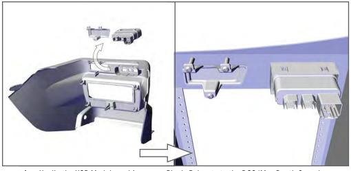
4. Unclip the USB Module and Accessory Blank. Relocate to the DGS/Max Depth Console by snapping the USB into place and secure the Blank with provided hardware.
