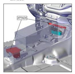
Place Console into the vehicle. Secure the Rear Mounting Bracket to the Console with previously removed OEM hardware, and the Front Mounting Bracket to the Console with provided hardware.
