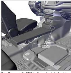
Remove (4) OEM bolts and retain for later use. Set OEM Floor Plate aside.
