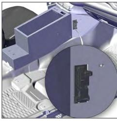
11. Attach the Manual Park Release (MPR) the side of the Console with provided hardware.
