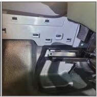
Move the DS/PS seats to the back position giving access to the OEM 10mm screws located in the sides of the center console.
