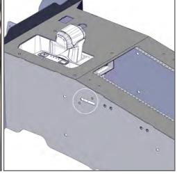
15. Place the OEM harness into the Contour Console. Plug in the collapsible shifter, and the proximity sensor. Secure the proximity sensor to the threaded studs located inside the Console. Use previously removed hardware for this step. (*REF STEP 9*)
