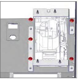
13. Attach the collapsible shifter to the Shifter Bracket with previously removed hardware. Once secure, transplant the assembly to the Contour Console and secure with (6) Flange Nuts.
