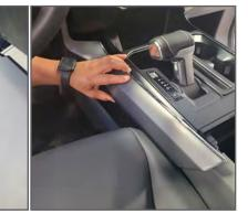
From the D/S of the console. Locate and remove the 7mm OEM screw securing the lower forward trim. Once removed, pull to unclip lower trim section followed by the upper trim section.
