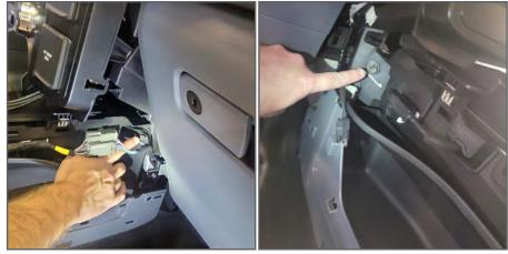
Remove the (2) OEM 10mm screws located on upper front of the center console attaching to the lower dash.
