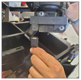
Unclip the consoles cup holder from its location. Unplug the proximity sensor and hardware. Set aside.
