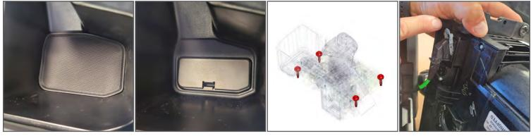
8. Pull out the rubber insert in front of the collapsible shifter exposing a removable plastic tab. This gives you access to the (2) of the (4) OEM screws. Once removed disconnect the OEM harness and **set aside**.
