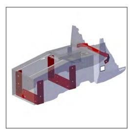
14. Place the Contour Console into the vehicle. Secure the Console to the installed brackets and secure with provided Socket Head Cap Screws (10) places. Secure lower front with previously removed OEM hardware. (REF Step 3)
