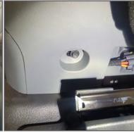
Move the DS/PS seats to the forward position. Remove the exposed OEM 10mm screws.
