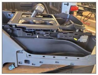
Remove the console from the vehicle and take to a location where further disassembly can be performed. Pop loose the (6) clips of the consoles top trim to remove the cup holder and shifter.
