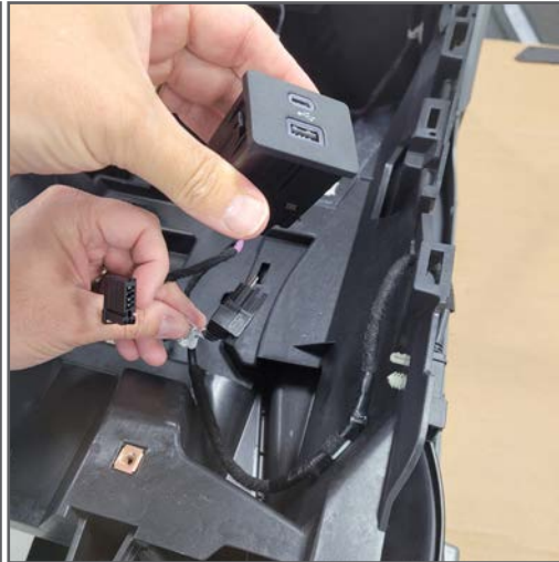
11. Fully remove the OEM harness from the center console. Unclip and disconnect accessories as you proceed.
