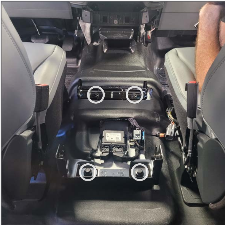
12. Remove the (4) 18mm bolts attaching the console's OEM brackets to the floor. With previously removed OEM hardware, secure the provided (2) Console Mounting Brackets in their place, followed by the Front Support Bracket with previously removed (10mm screws from REF Step 5)
