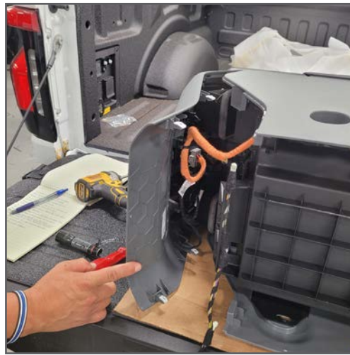
10. Place the center console on its side and pop loose the rear trim. Unplug and remove the USB and 120v power plugs.
