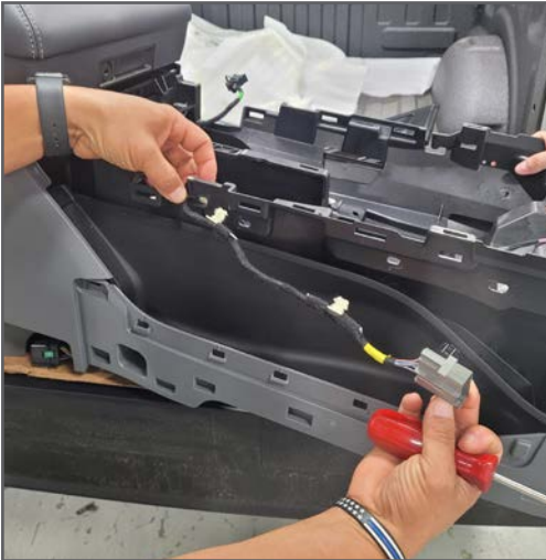
9. Unclip the console's cup holder from its location. Unplug the proximity sensor and hardware. Set aside.
