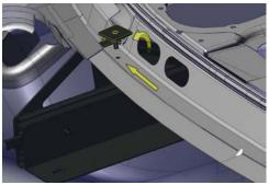
Place the mounting plates inside the openings in the underside of the rear deck lid, (2) per side. With a friend, attach the front supports arms of the tray to the mounting plates previously installed using the  $\frac{1}{4}$ -20 flange nuts provided.
