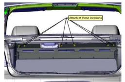
Install to the back of the trunk with the provided self-tapping screws. Drill (6) screws into the back of the trunk.
