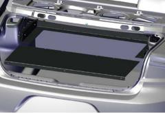
With the trunk tray secured front to back, mount all hardware / equipment to the detachable slide tray. Slide back into place and secure with (6) flange nuts in the back and (2)  $\frac{1}{2}-20x^{3}/4$  carriage bolts.
