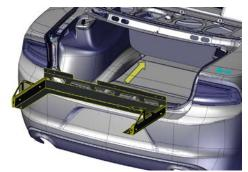
Remove the detachable tray from the trunk tray. Slide the Trunk Tray assembly in the car and check for proper placement.
