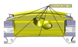
Remove the insulation panel on the underside of trunk deck by pulling out (5) press-in plastic pens in the body of the panel and (2) on the sides.
