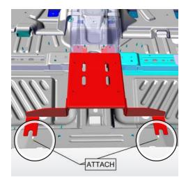
Attach the rear left and right legs of the Mounting Base to the underside of the rear seat with OEM hardware.
