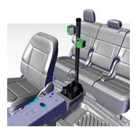
5. Attach Backbone assembly to top of Mounting Base using (4) provided 1/4" x 20 x 3/4" button head cap screws
