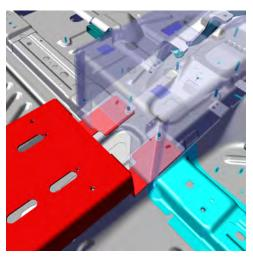
Loosen the (2) rear OEM Cover Plate Bolts and slide the Mounting Base under.
