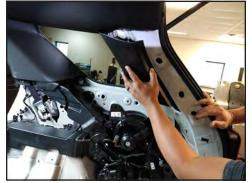
10. Pull the rear upper "D" pillar trim up and out to unclip from its location.
