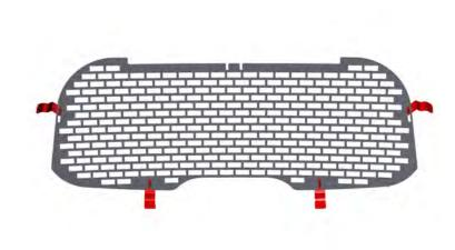
20. Lightly secure the remaining mounting brackets to the Rear Window Armor with provided ¼-20 flange nuts.
