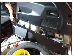
7. Remove the LH/RH lower side panel by using a small flat head screwdriver to pop up the center of the press in plastic pins. (14 per side)
