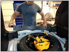
6. With a trim removal tool pry, around the edges of the rear lower cargo trim to separate it from the cargo compartment.
