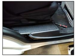
11. With a trim tool pop up the lower door trim panel. Remove the (2) press in pins holding the panel to the lower seat skirt fabric.
