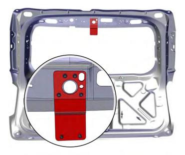
19. Attach the Top Center Bracket to the rear deck lid by aligning the circular profile, secure in place with self-tapping screws.
