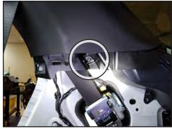
12. Remove the screw located on the bottom of the DS/PS "C" panel trim using an 8 mm socket.
