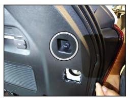
8. Unscrew the LH/RH accessory hatch cover pins with a pair of pliers.
