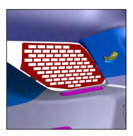
17. With the Window Armor attached, reinstall all previously removed side trim to complete assembly.
