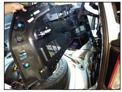
Start at the rear to remove the P/S upper side panel with a trim removal tool. Pull out far enough to unplug the cargo light and 12V power supply.
