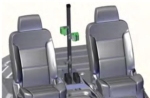
Position assembled backbone onto GR6 mounting plate.
