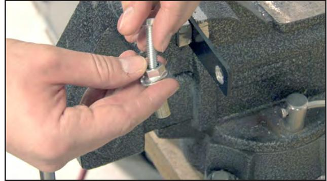
2. Place 5/16-18 x 1.5" long bolt through the 3/8" flange nut and hand thread bolt into the AVK Fastener.
