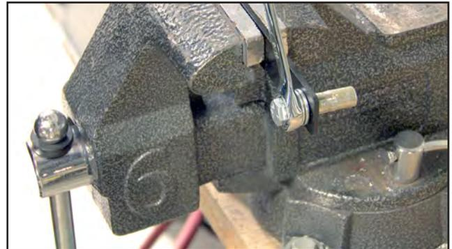
4. Use 9/16" box end wrench to secure the flange nut.
