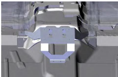
Reposition mounting plate underneath seat rails of front seats and tighten all OEM seat bolts and use provided hardware for AVK locations.
