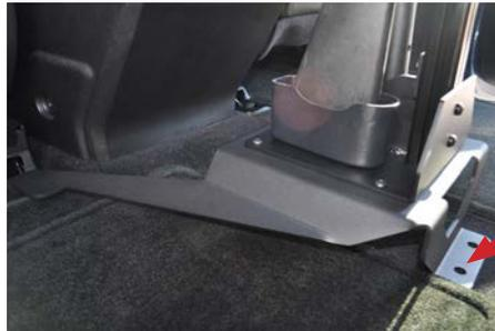
Slide GR6 mounting plate on top of inside seat rails of front seats. Mark hole location for rear of mounting plate for AVK install. Remove mounting plate and set aside.
