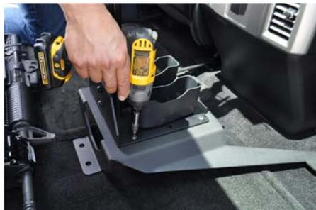
Position assembled backbone onto GR6 mounting plate.
