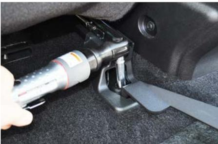
Reposition mounting plate on top of rear seat rails of front seats and tighten all OEM seat bolts and use provided hardware for AVK locations.
