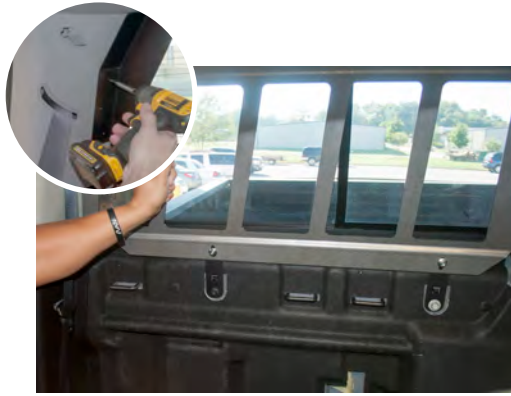
Secure Rear Window Armor to all brackets using provided (3) flange nuts on Lower Brackets and (6) tek screws on Side Brackets. Once Window is in position, tighten all hardware.
