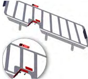
Attach the Upper and Lower Center Mount Brackets to the Window Armor with the provided hardware.
