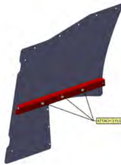
Outside of the vehicle, attach Lower Stiffener Tube to Lower Center Divider on driver side.
