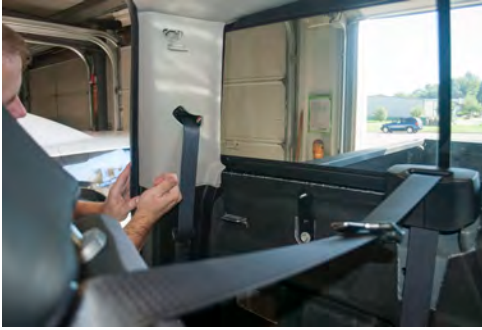
Replace OEM "C" pillar trim and tighten the (3) Lower Brackets
