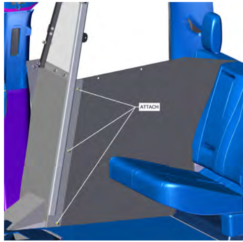
11. Loosely secure Lower Steel Center Divider onto Assembled Front Divider using provided carriage bolts and flange nuts.
