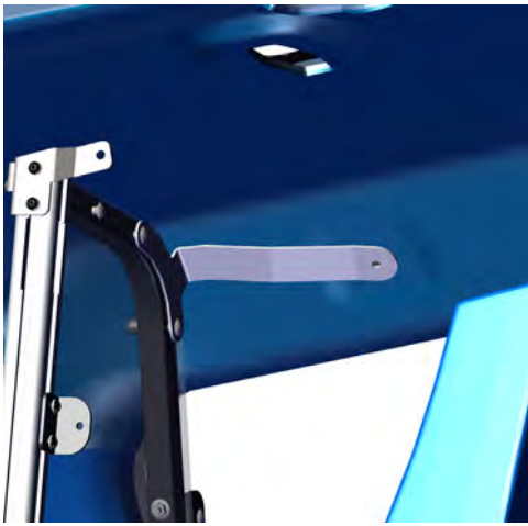
10. Loosely attach Headliner Handle Bracket into grab handle location. Reuse OEM bolts.
