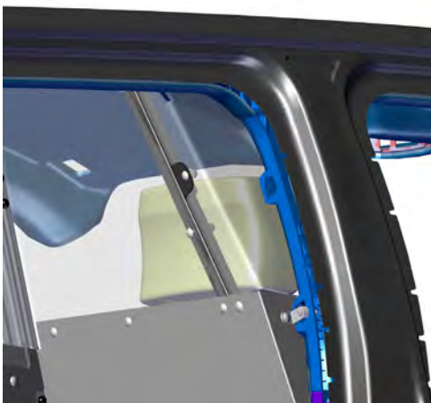
16. Install Upper Poly Wing from front of vehicle using provided carriage bolts and flange nuts.
