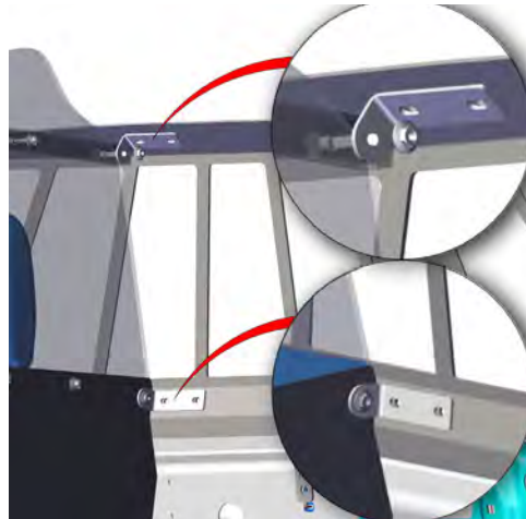
14. Attach Upper Mount Bracket to Upper Poly Center Divider and Lower Mount Bracket to Lower Steel Center Divider with carriage bolts and flange nuts.
