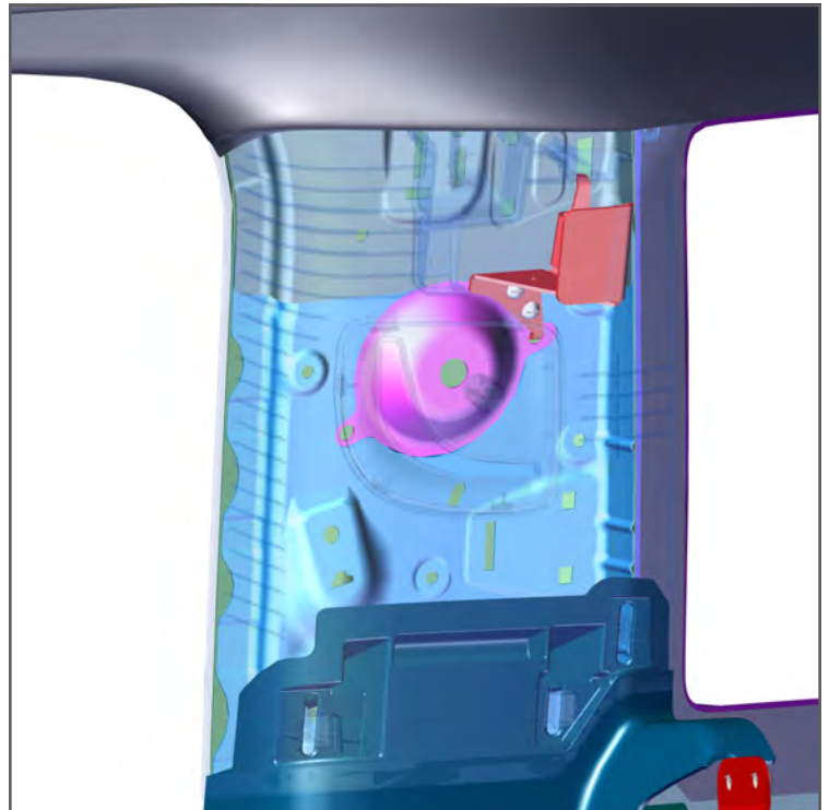
7. Replace OEM "C" Pillar Trim on top of P/S Side Armor Upper Brackets. REPEAT FOR OTHER SIDE.
