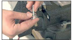
Place 5/16-18 x 11/2" long bolt through the 3/4" flange nut and hand thread bolt into the AVK Fastener.
