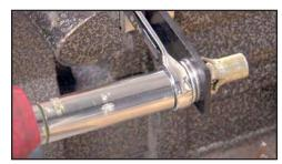
Apply pressure on the flange nut, pressing AVK Fastener into hole.
