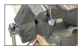
4. Use %6" box end wrench to secure the flange nut.
