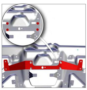
7. With AVK Fasteners installed, re-attach the GR4 Mounting Plate to the Rear Deck Lid with provided  $\$_{16}\text{-}18~x~1"$  bolts and secure.
