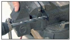
Drill out existing hole to ½" or drill new hole per installation instructions.
