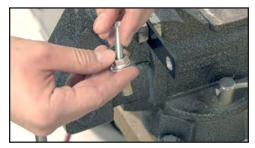
Place %-18 x 1½" long bolt through the %" flange nut and hand thread bolt into the AVK Fastener.
