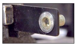
This will allow the AVK Fastener to secure onto the backside of the metal.
