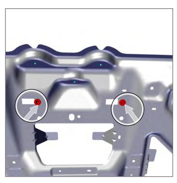
3. Locate the (2) factory holes on the Rear Deck Lid and install provided AVK Fasteners. Holes need enlarged to  $1\!\!/\!\!2$  diameter.
