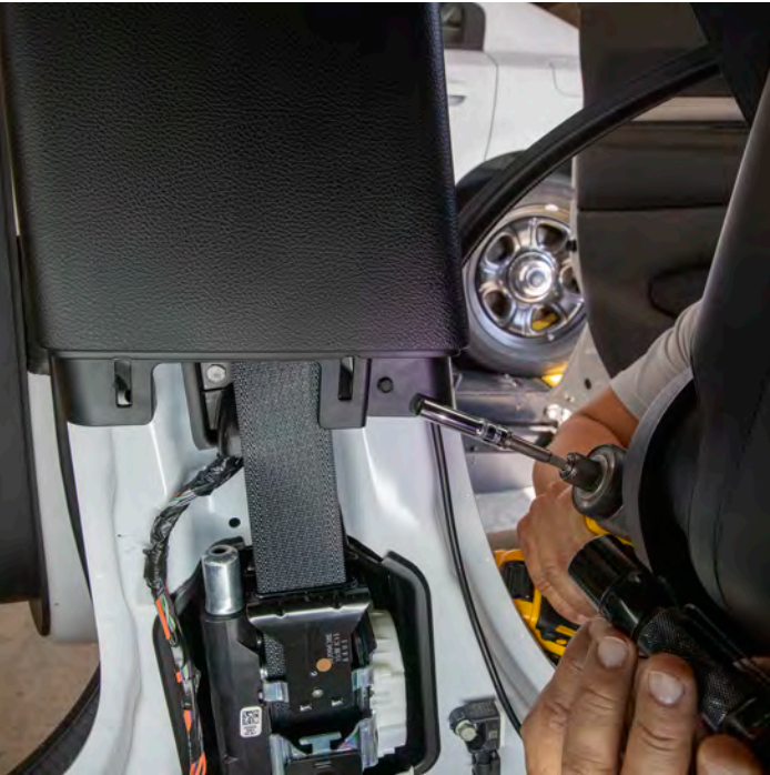
3. Using 3/2 socket remove exposed screw from upper B-Pillar trim. Remove upper B-Pillar trim.
