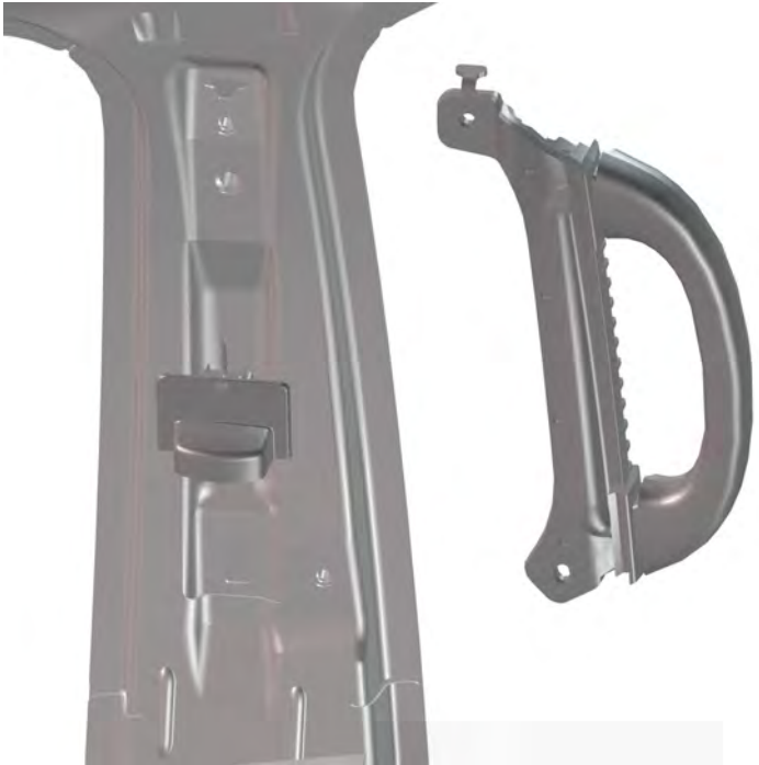
4. Use a 10 mm socket to remove both OEM bolts and grab handles. NOTE: PART NOT REINSTALLED
