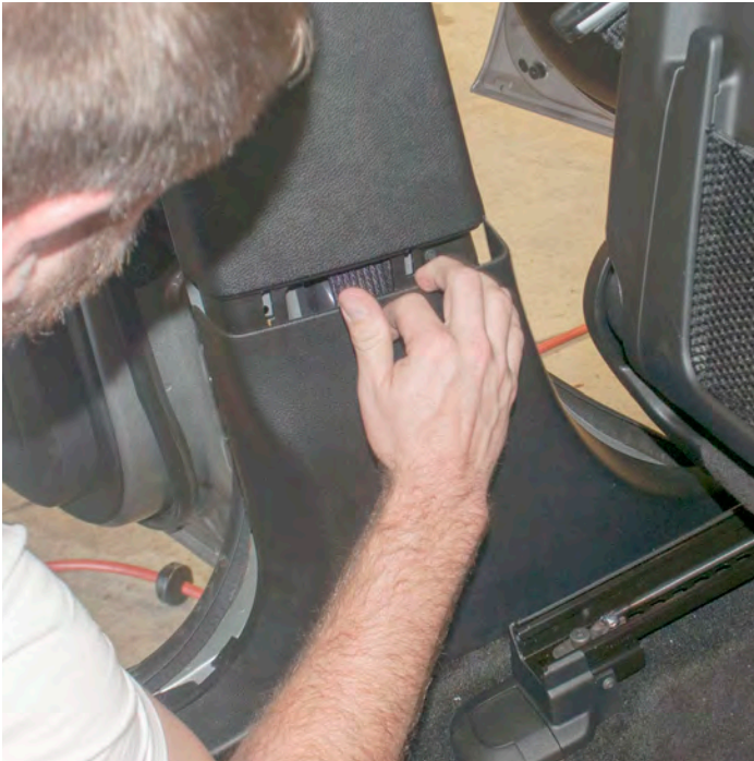
2. Pop plastic clips and remove lower B-Pillar trim.
