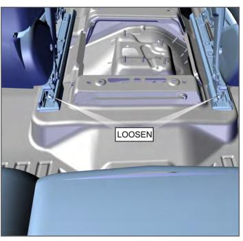
Move front seats completely forward and loosen the rear inside T-50 bolts.
