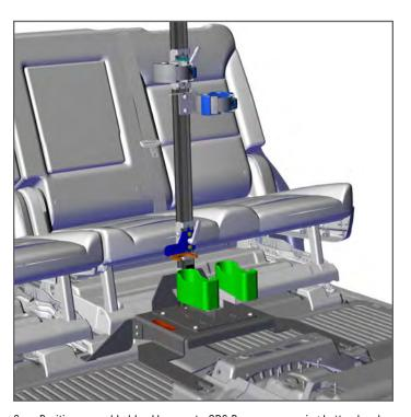
Position assembled backbone onto GR6 Base, secure using button head cap screws. Secure all hardware and previously removed plastic trim.
