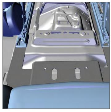
3. Push the seat up slightly to slide the front legs of the GR6 Base under seat rial, between rail and vinyl/carpet flooring.
