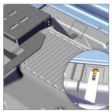
5. Hold the D/S Rear GR6 leg to the side of the GR6 Base. Measure and mark out where to cut out a 3"x3" section of the carpet/vinyl, giving access to the OEM threaded hole. Secure GR6 Leg with provided M10-1.5x50 bolt and to the GR6 Base with button head cap screws.
