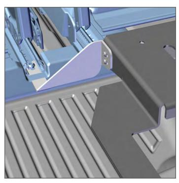
Loosen the rear seat inside T-50 bolt and insert the P/S Rear GR6 Leg between the rail and flooring. Secure the Leg to the GR6 Base with provided button head cap screws.
