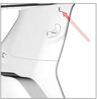
. Remove the upper C-Pillar trim by popping out square trim cover, giving access to the 9/32" screw at the top of the headliner.
