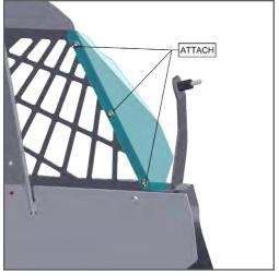
Attach the DS/PS Side Poly Wings from prisoner side with (6) 1/4-20 carriage bolts, 1/4" flange nuts and nut cover.
