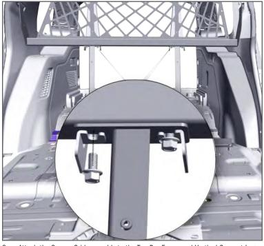
Attach the Secure Grid assembly to the Top Bar Frame and Vertical Support Legs with provided (4)  $3/8 \times 3/4$  hex head bolt.
