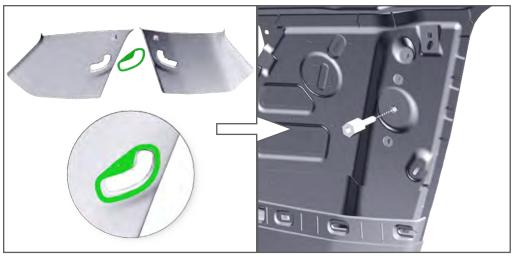
3. Using provided drill template (P21T60DT), drill 1/8" pilot hole into C-Pillar trims, follow up with 1-1/4" hole saw to cut out plastic trim. Remove upper C-pillar seat belt bolt and replace with Seatbelt Standoff Bolt. Roll up seat belts and secure with zip ties and reinstall C-Pillar trim.
