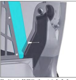
Attach the DS/PS Wing Covers to the Top Bar Frame with provided (2) 1/4-20 x 3/4" button head cap screws.
