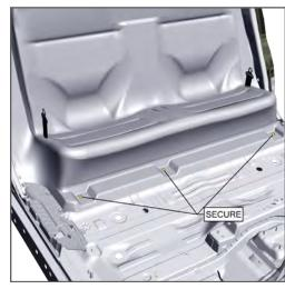
Secure the front of the ABS Seat with previously retained OEM seat hardware.
