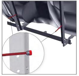
18. Thread (2) 1/4-20 x 5" all thread into the top hole and secure in place with a 1/4-20 nut from the back side.
