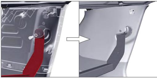
Install Top Bar Frame through the DS/PS seatbelt slots using provided (2) 7/16 x 1" hex head bolt and (2) external tooth lock washer.
