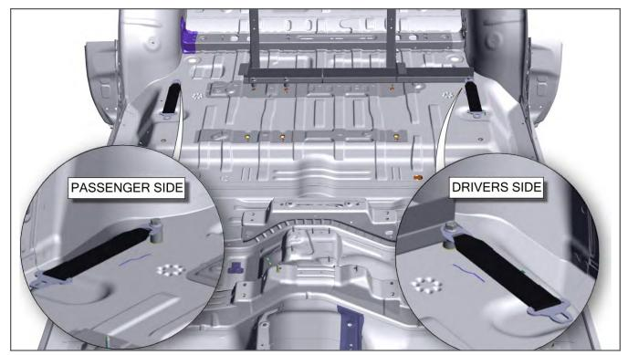
Attach the Hip Side Tongue Belts with provided (2) M10 x 50 mm bolts and (2)-spacers. Driver side will be on top of the Lower Vertical Support Bracket and passenger belt will be located at the rear outer most passenger seat bolt location.
