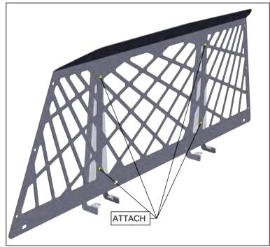
7. Attach the Support Grid Brackets to the Secure Grid with (4)  $1/4-20 \times 1/2$ " button head cap screws.
