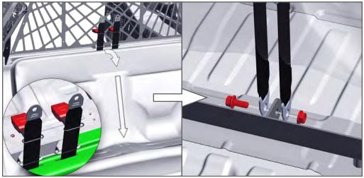
13. Pull the ends of the Seat Belt Retractor through the top slots of the ABS Seat and put the ends of the Seat Belt Retractor through the Seat Belt Sliding Buckles. Pull the Retractor Belts through the middle of the ABS Seat slots and secure to the tab of the Lower Support Bracket with provided 7/16-20 x 1" flanged hex bolt and 1/16 hex nut.
