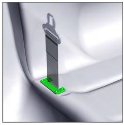
Attach the Toothed C-Retainer around DS/PS seat belt and secure to the ABS Seat with (8) #6 x 5/8 sheet metal screws.
