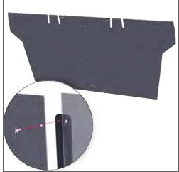
Outside of the vehicle, attach ABS Cargo Cover together to the center support with (6) 1/4-20 x 3/4" socket head cap screws and 1/4" nuts.
