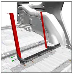
5. Install DS/PS Vertical Support Legs using provided (4) 3/8"-16 x 5/8" bolts.
