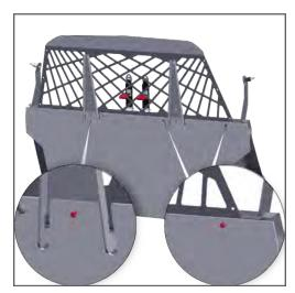
20. Place the assembled ABS Cargo Cover into the vehicle. Adjust the threaded studs as needed to give proper clearance when attaching the Cargo Cover. Secure the Cargo Cover to the Top Bar Frame with provided (2) #14 x 1" tek-screws and (4) 1/4-20 x 1/2" flanged hex head cap screws.
