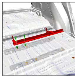
Loosely install Lower Support Bracket using provided (2) M10 x 50mm bolts and (2) spacers.
