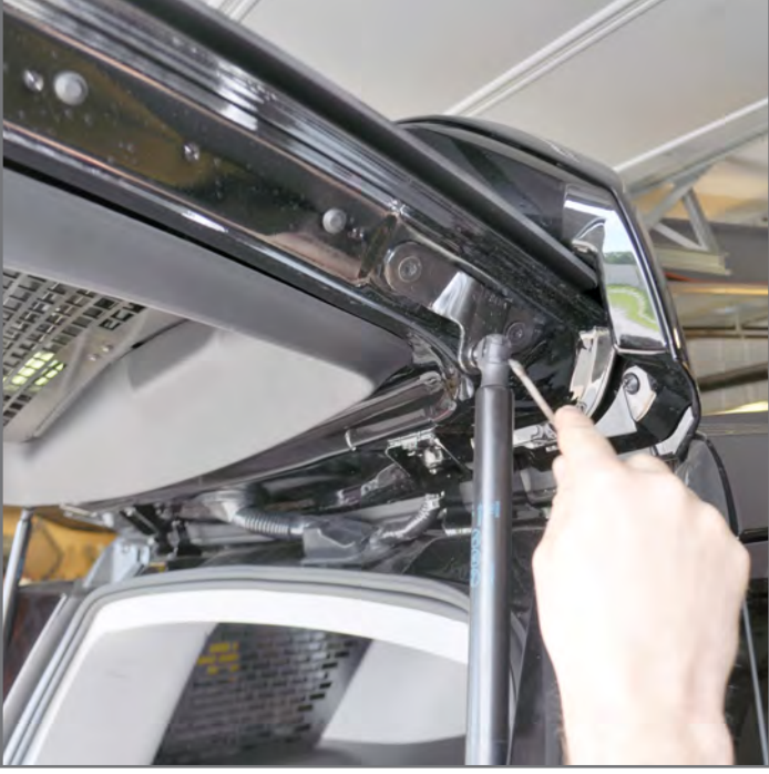
8. Remove OEM strut by using a flat head screwdriver. Slide the screwdriver under the clip and pry away from strut. Then proceed to pull strut away from OEM frame.
