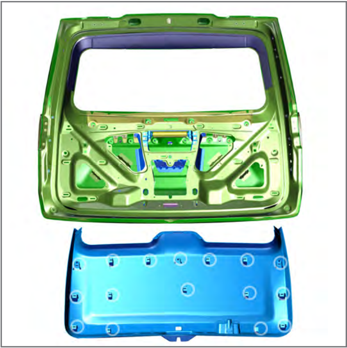
2. Once screw is removed, carefully remove the lower OEM hatch trim by prying at the edges unclipping from its (15) locations.
