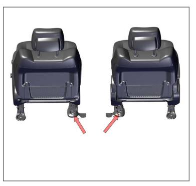
1. With a small screwdriver, unsnap the inside rear seat trim (of the front seats) exposing the OEM seat bolts. Remove with a 15 mm socket.
