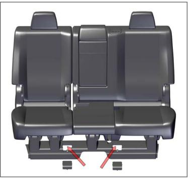
2. With a small screwdriver, unsnap and set aside the rear seat trim covers exposing the OEM seat bolts. Remove with a 18 mm socket.
