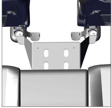
4. Replace and tighten OEM bolts to secure GR6 mounting plate.
