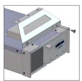
Attach the (2) Cargo Cover Brackets to the tabs found on top of the "Stash" Gun Boxwith (4) 5/16-18 socket head cap screws. NOTE: 3/16" Torx Socket Bit required
