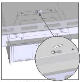
Loosely attach (1) socket head cap screw to the center hole of each previously attached Cargo Cover Bracket. Install the Gun Box under the Cargo Cover, lift-up into the Cargo Cover exposing the screw within the hole-slot. Slide over to hold in place.
