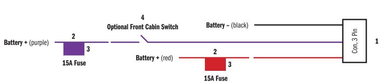
\* - Battery connection can be Switched or Constant basted on the desired function. Ignition **ON** or **OFF** function.
