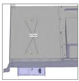
Attach the remaining (4) Socket head cap screws through the Cargo Cover to securely attach the Gun Box into place.
