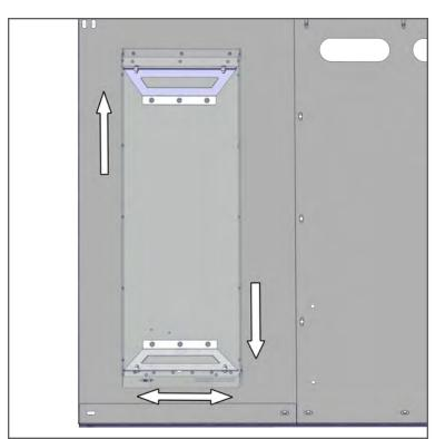
Adjust to desired location and mark points to drill through the (6) mounting holes located on the Cargo Cover Brackets.
