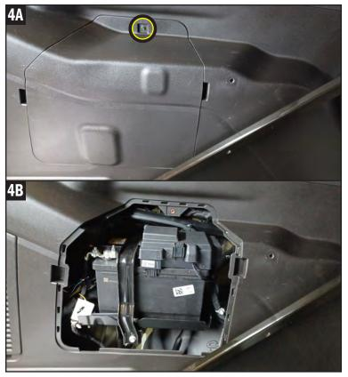
Remove the screw and pop loose to remove the battery cover.
