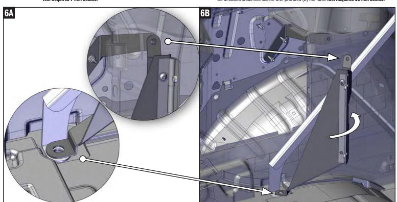
6 Remove the bolt securing the Cargo Barriers Rear Mount Leg, place the Gun Box Bracket on top and loosely attach. Rotate the Gun Box Bracket to the trim aligning the mounting point of the Inner Trim Bracket. Mark a drilling point, rotate the bracket away to drill a ¼" hole.
