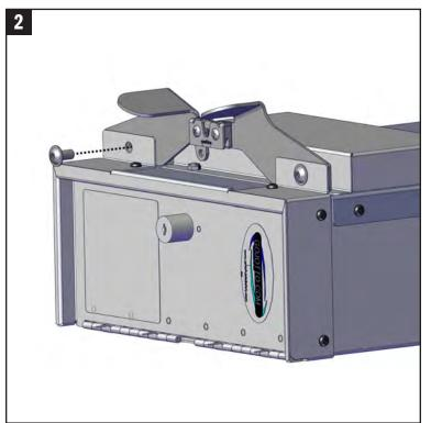
2 Attach the Latch Bracket to "The Stash" Gun Box with provided 5/16"-18 socket head cap screws. **Tool Required 3/16" Torx Socket**
