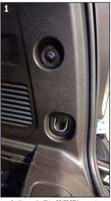
Unscrew the (2) top DS/PS OEM cargo net hooks, along with the bottom ring hood supports. Tool Required, TP-40 Socket
