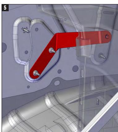
With or without the vehicle's battery removed, place the InnerTrim Bracket on the exposed OE threaded studs and secure with provided (2) M6 nuts. Tool Required 10 MM Socket.
