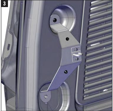
3 Attach the Striker Bracket to the cargo area. Secure the top hole with provided hardware M6-1" socket head cap screw, and the bottom with previously removed screw. Tool Required T-27 Socket Bit
