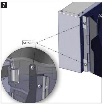
7 Secure the Box Bracket to the InnerTrim Bracket and the Gun Box with provided (4) 5/16"-18 socket head cap screws. Finish by attaching Gun Box to the Box Hinge and Latch Bracket.
