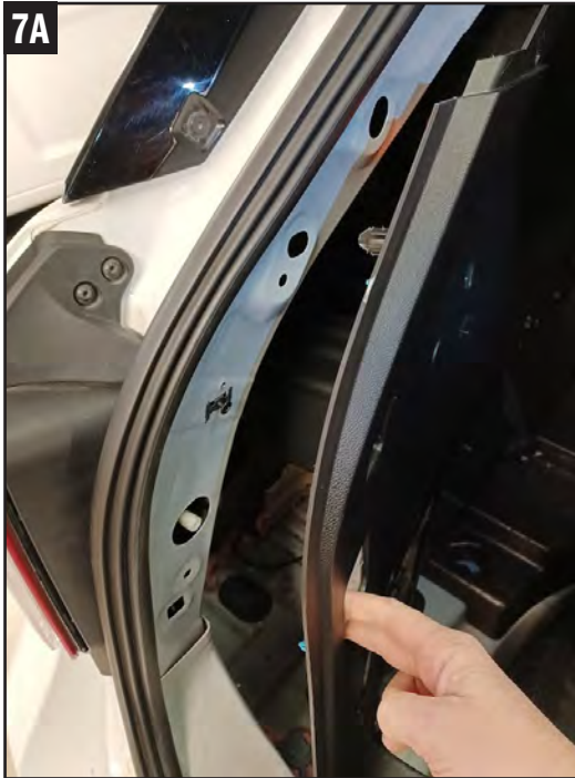
7 Starting from the cargo area, pop loose the upper panel while moving forward to the rear seat area. Once loose, remove from vehicle.
