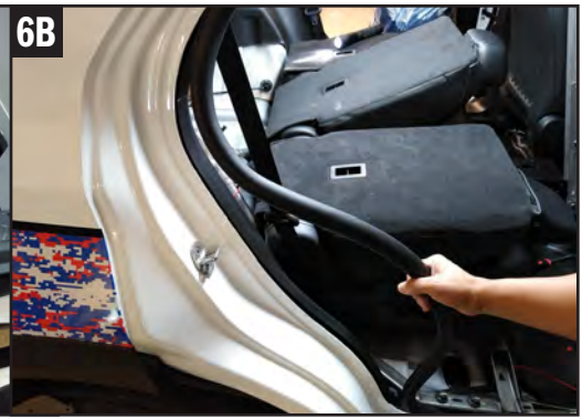
6 · Pop loose the (2) press in pins holding the panel to the lower seat skirt fabric, remove trim section. · Fold the rear seats down and pull the rubber door seal away from the "C-Pillar" side panel.
