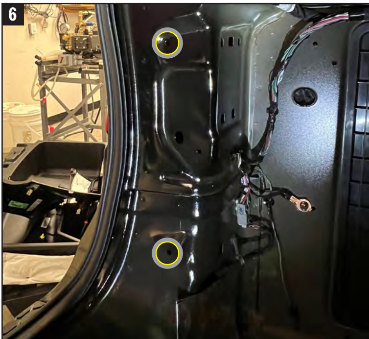
6 Install the (2) provided AVK fastener in the mounting location of the previously removed clips. FOLLOW AVK INSTALLATION INSTRUCTIONS ON PAGE 4.
