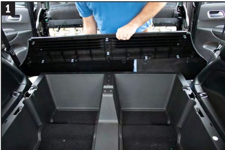
**1** Remove lids from the storage compartment by opening them 90° and pulling at an angle to unclip from three positions (EACH SIDE). You will also have to remove the front trim portion from the storage box by pulling at an angle releasing (8) clips.
