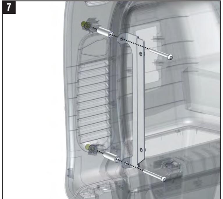
**7** Secure the Front Stash Bracket to the previously installed AVK fasteners with (2)- Gun Box Spacers and 5/16"-18 x 3-1/4" button head cap screws.
