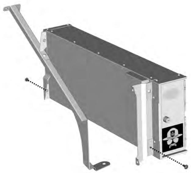
9 Complete assembly by attaching the Gun Box to the Front/Rear Brackets with (4) 5/16"-18 socket head cap screws. Fully secure all hardware at this time.
