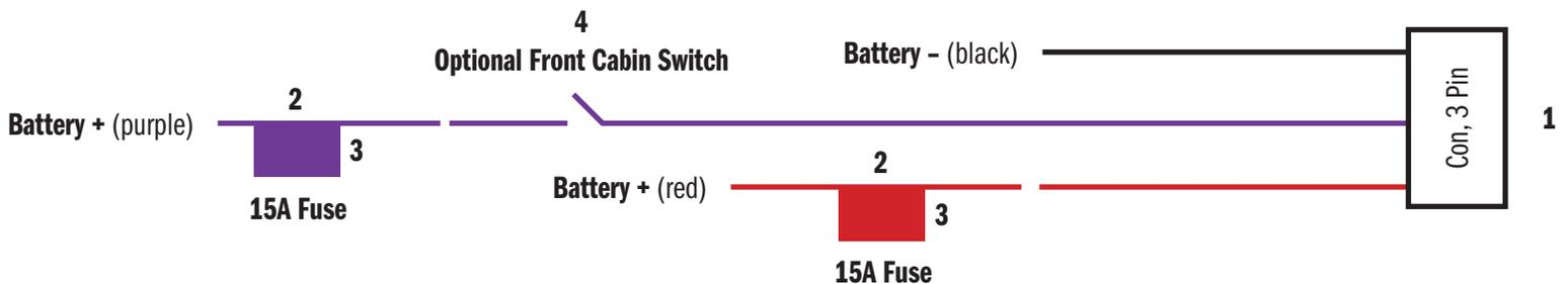
\* - Battery connection can be Switched or Constant based on the desired function. Ignition **ON** or **OFF** function.
