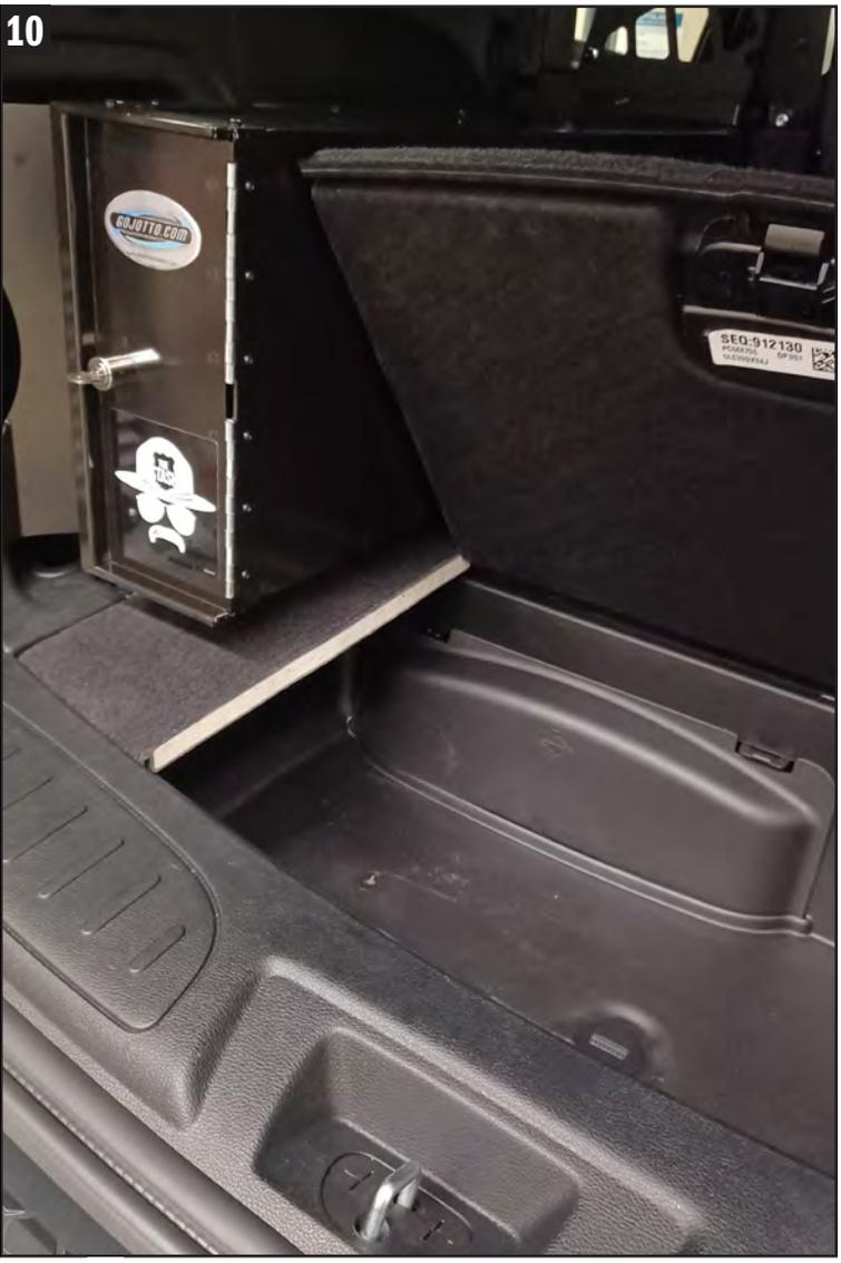
10 Mark lid/cover for cutting in order to gain access to spare tire/jack/etc. Remove lid/cover, cut and replace.
