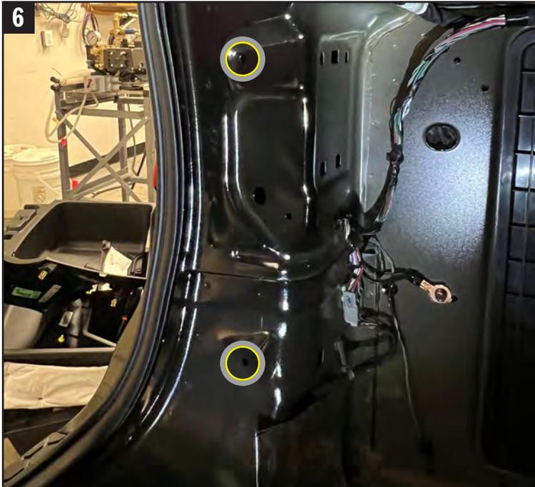
**6** Install the (2) provided AVK fastener in the mounting location of the previously removed clips. **FOLLOW AVK INSTALLATION INSTRUCTIONS ON PAGE 3.**
