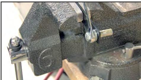
4. Use 9/16" box end wrench to secure the flange nut.
