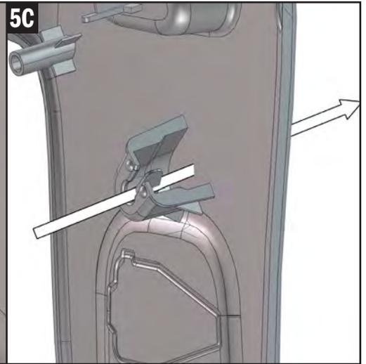
**5** Remove the (2) clips that secure the trim. Cut the tab away from the trim support. Use the circular profile of the interior trim support to drill a 9/32" hole through the trim followed by a 3/4" inch hole.
