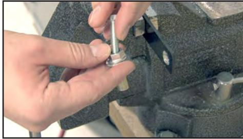
2. Place 5/16-18 x 1.5" long bolt through the 3/8" flange nut and hand thread bolt into the AVK Fastener.
