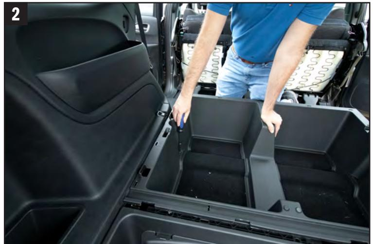
**2** Remove the (2) 9/32" screws removing the storage compartment.
