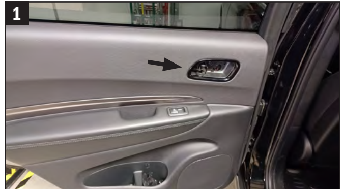
1. Remove the Latch Cover and Handle Cover to gain access to the OEM hardware. 10 mm Socket / Phillips required.
