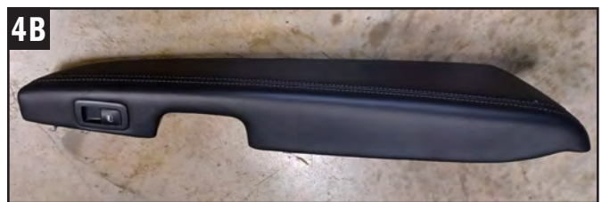
4. Remove the (16) screws from the back side of the door panel, removing the armrest section from the panel. Torx-15 Socket required.
