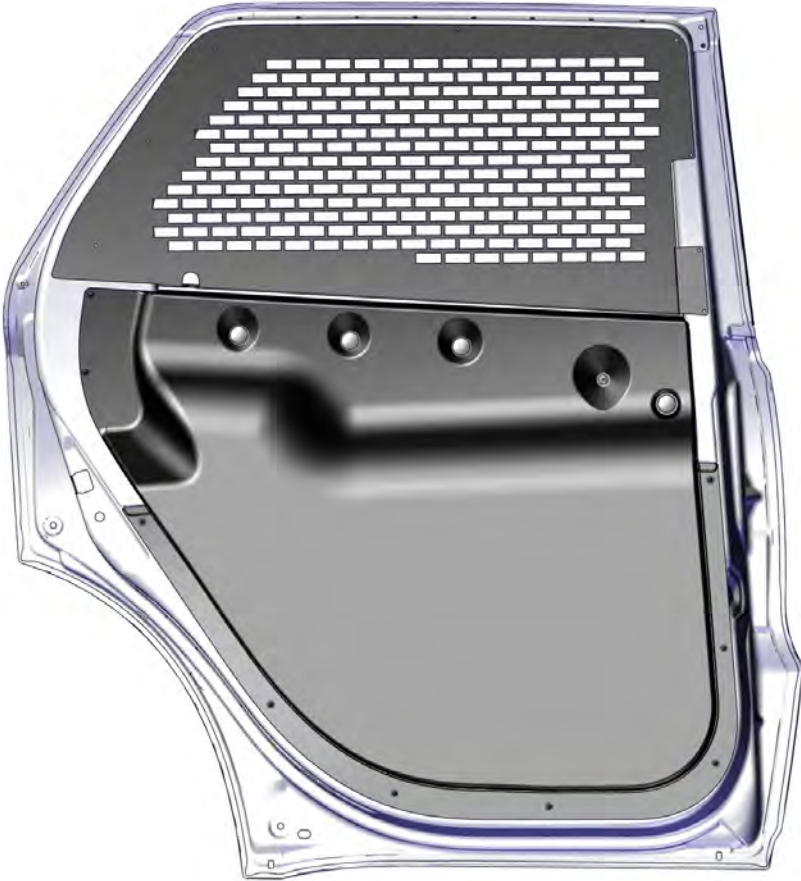
1. Remove the Latch Cover and Handle Cover to gain access to the OEM hardware. 10 mm Socket / Phillips required.
