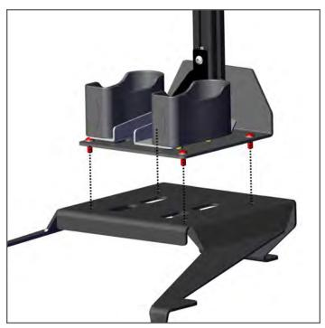
4. Reposition mounting plate under the seat rails and tighten all OEM seat bolts, replace trim cover and use provided hardware for AVK locations.
