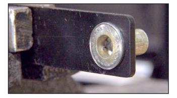
7. This will allow the AVK Fastener to secure onto the backside of the metal.
