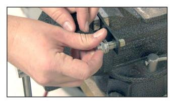
Place into 1/2" drilled hole.
